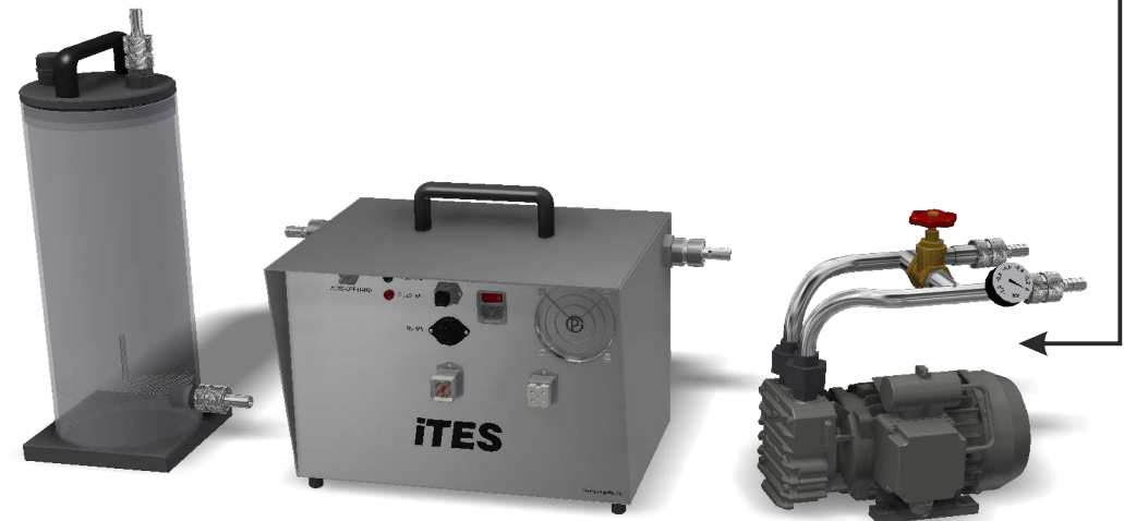
Absaugung: Trockenturm, ITES und Pumpe suction line: drying tower, ITES and pump
